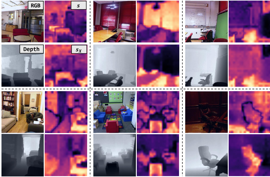
Fig. 9: Qualitative analysis of the Cross-modal Harmonization. The figure displays the RGB image, the shared representation s , the auxiliary Depth modality, and the modality specific proxy s_X . This comparison highlights how s_X serves as a tailor made bridge for CMCS loss calculation, ensuring that s maintains rich semantic information while achieving robust alignment with the depth structure.
